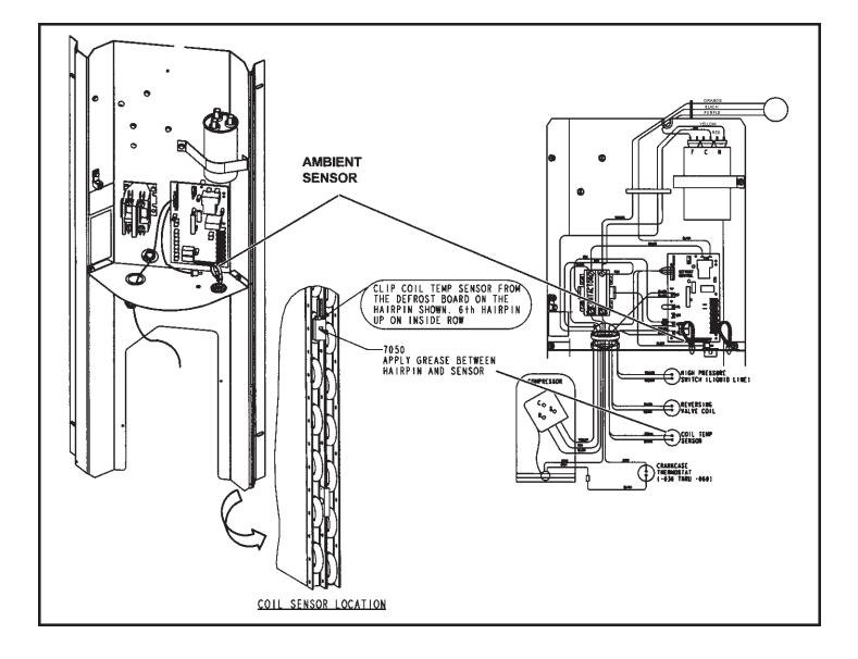
Ambient Sensor—The ambient sensor considers outdoor temperatures below -35°F (-37°C) or above 120°F (48°C) as a fault. If the ambient sensor is detected as being open, shorted or out of the temperature range of the sensor, the board will not perform demand defrost operation. The board will revert to time/temperature defrost operation and will display the appropriate fault code. Heating and cooling operation will be allowed in this fault condition.
